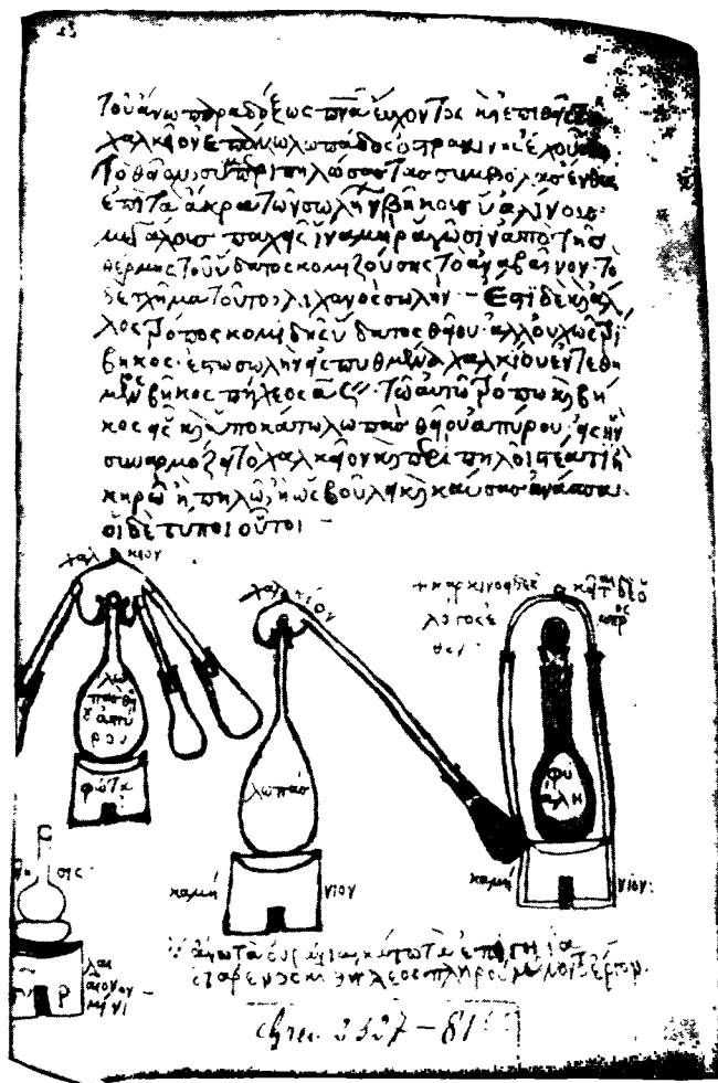
FIG. 3.—THESE DRAWINGS ILLUSTRATE TYPES OF APPARATUS FOR DISTILLATION AND SUBLIMATION CLOSELY RESEMBLING THAT USED IN CHEMICAL WORK UP TO THE CLOSE OF THE EIGHTEENTH CENTURY. (MS. PARIS, GR. 2327, F. 81.)
